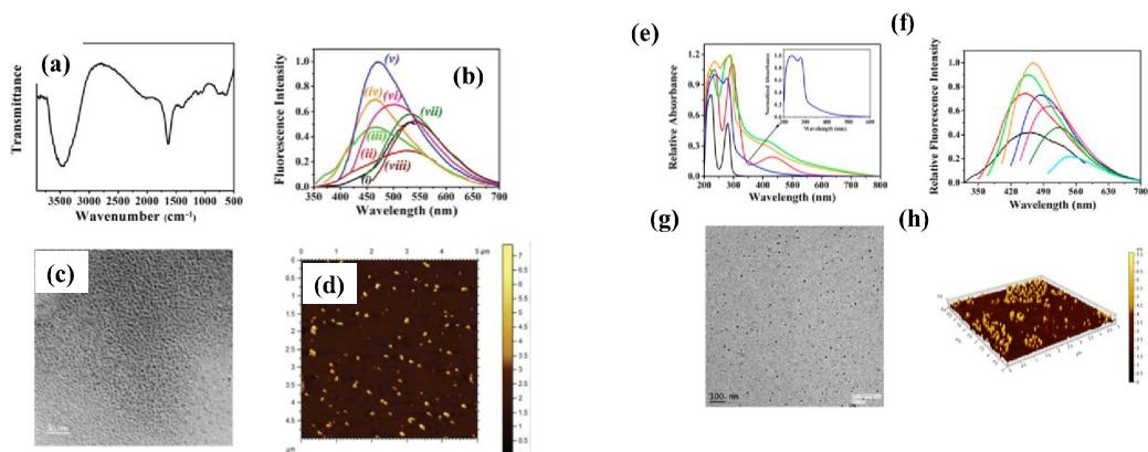
**Figure 1.** Spectroscopic characterization using (a) FT-IR, (c) steady-state emission (i, ii, iii, iv, v, vi, vii and viii indicate emission spectra corresponding to 280, 300, 330, 350, 375, 400, 420 and 440 nm excitation wavelengths, respectively) spectra and microscopic analysis employing
