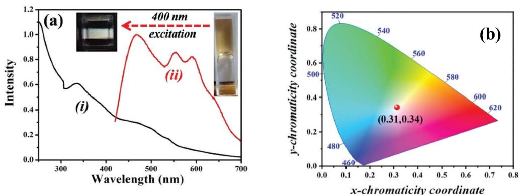
**Figure 5.** (a) UV-visible absorption (i) and steady-state emission (ii) spectra with the inset shows the digital micrographs of WL@agarose gel under day light and 400 nm excitation light; (b) CIE plot for the CD–Dox WL system in agarose gel. Figures (a–d) are reproduced with permission from ref 19 (Copyright 2019 Royal Society of Chemistry).
