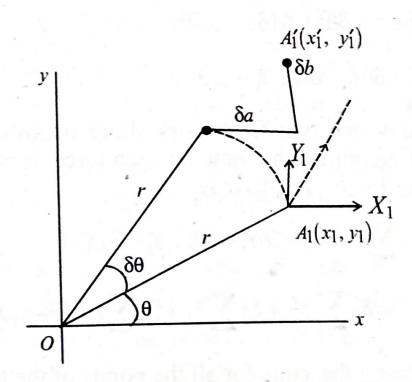
Now, when the body receives a small virtual displacement consistent with the geometrical conditions of the system, the point  $A_1$  takes the new position  $A_1'(x_1', y_1')$  by two type of motion: one due to rotation through a small angle  $\delta\theta$  and other due to translation through small distances  $\delta a$  and  $\delta b$  parallel to co-ordinate axes.
