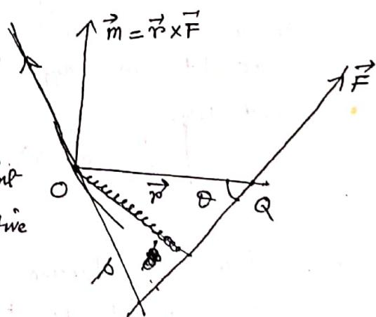
Note: (i) We define the projection of  $\vec{m}$  on  $\vec{b}$  as the moment of the force  $\vec{F}$  about the line  $\vec{b}$ . Thus, the moment of  $\vec{F}$  about the line  $\vec{b}$  is given by
